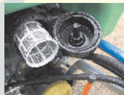
Easy inspection suction filter
